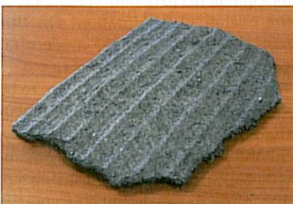
Figure 6. Peeled-off slag layer
